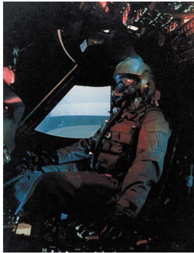
Figure 3: The helicopter flight simulator simulates the UH-60, being fully instrumented with six degrees of freedom in motion and fully visual display adjustable to day or night missions.
