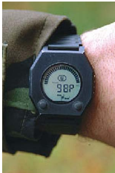
Figure 2: The Actigraph is a wristwatch-like device that measure wrist movement which enables determination of an individual's sleep/wake cycle and consequently estimates fatigue level.
